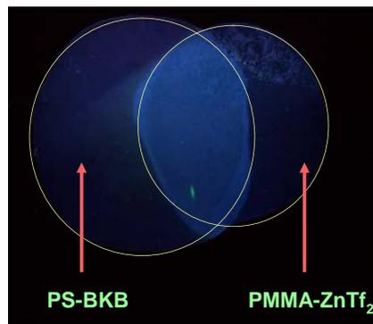
**Evidence of self-assembly between layers of PS and PMMA containing 1% w/w of macromonomer and zinc triflate, respectively (under UV light)**
