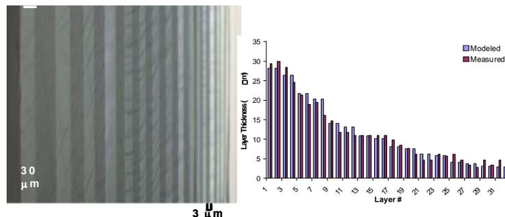
**Cross-section of a 32 layer PS/PMMA gradient layer film produced by ‘uneven’ split layer multiplication (left); and comparison of the measured and calculated layer thickness distribution (right)..**
