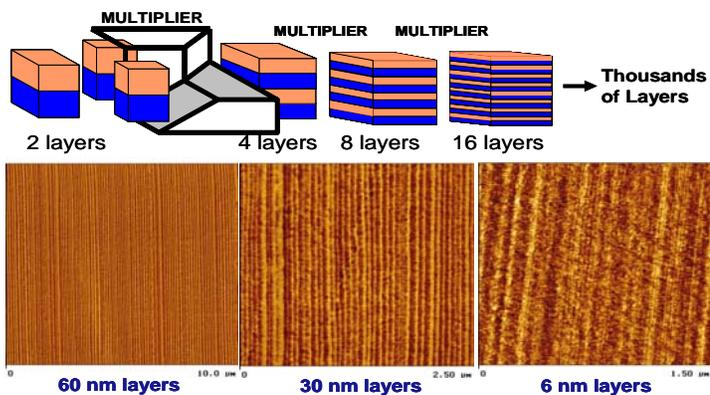
**Layer Multiplying Coextrusion Technology**
