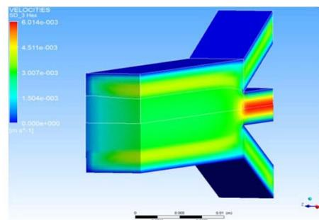
Velocity profile (in Polyflow) for half cut of the Feedblock
